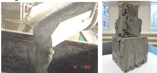
Cargo concrete - Cubic concrete samples tested at compression
